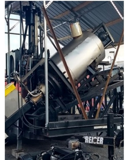
The inclined rotary gasifier developed at SCU (source: SCU).
